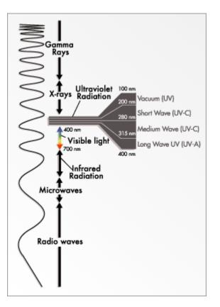
**Long-wave UV**, or UV-A, is the kind used in entertainment applications. This is what's known as "black" light. ("Black" because you can't see it.) In comparison to short-wave or medium-wave UV, long-wave UV is pretty safe. This range is defined by the wavelengths between 315 and 400nm. Remember that 400nm is about the extreme edge of visible light. So this range is just beyond what humans can see. So how is it we can see under black light? Well, there are two reasons.
