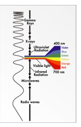
Wavelengths of electromagnetic energy between roughly 400 and 700nm (nm = nanometers, or *one billionth* of a meter) are visible to the human eye. The longer wavelengths—toward 700nm—are on the lower end of the visible spectrum, while the shorter wavelengths—toward 400nm—are on the upper end of the spectrum.
