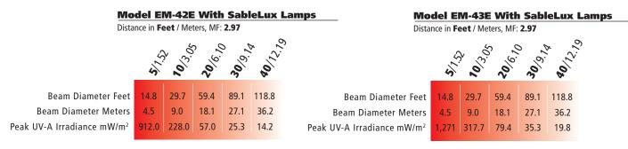
All peak UV-A irradiance measurements taken at center beam using UVX Digital Radiometer and a calibrated 365nm sensor
